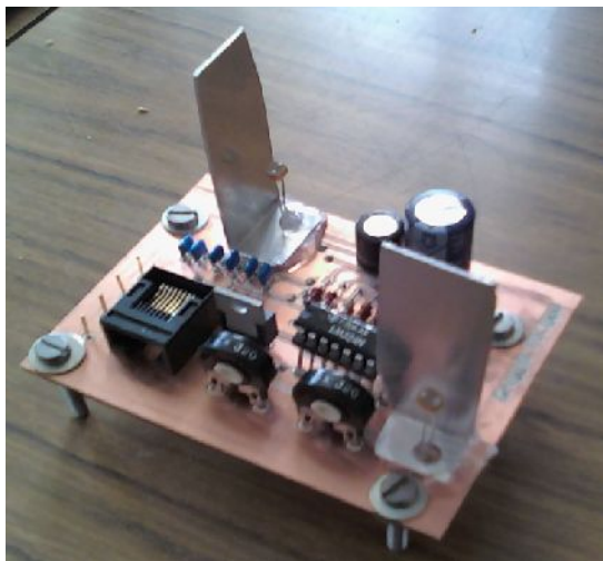
above: photo of the electronic board of the circuit that detects the position of the sun;
